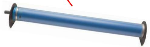
**With the 10 EW variant**, a 1070 mm long tube aerator is positioned on the tank bottom in the longitudinal direction of the tank (marking on the right). Enlarged spacers are mounted on this tube diffuser to prevent the membrane for the contact with the tank bottom.
