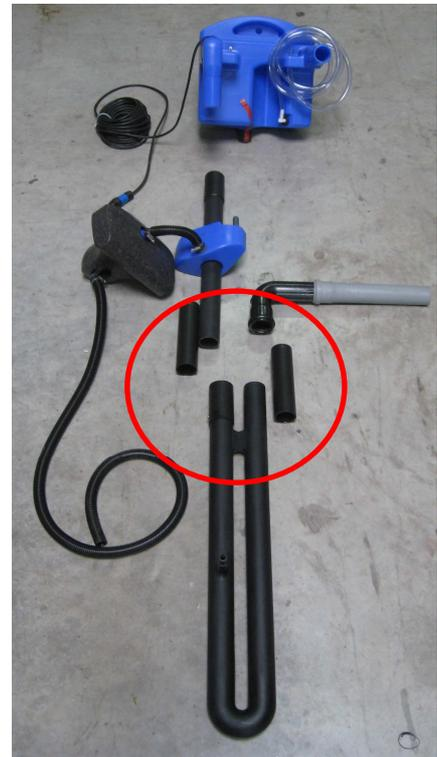
Assemble the pipe set as shown in the diag. right and secure the sleeve using the inserted screws.
