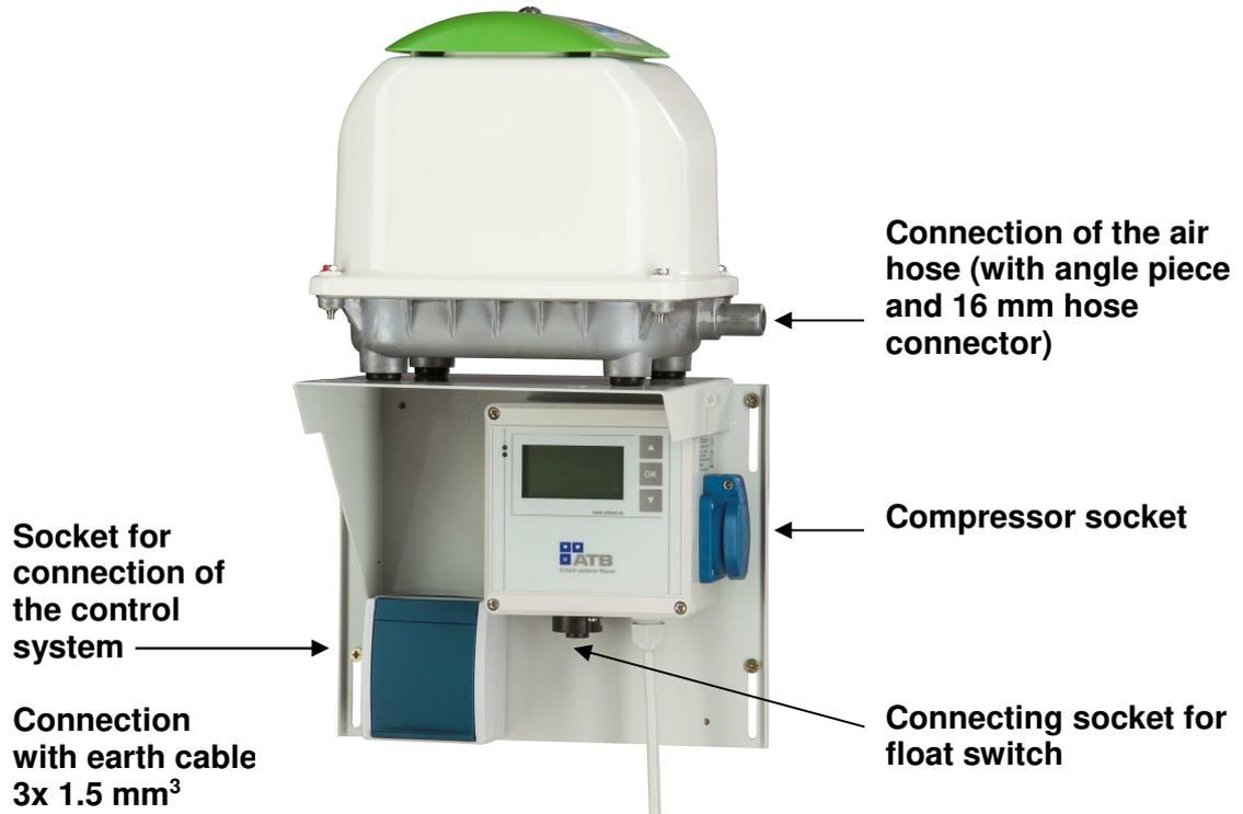
Install the control unit either directly to the console on a stable wall or in the cabinet which can be supplied as accessory (inside cabinet/open air column). The maximum separation between tank and mounting location of the control unit may not exceed 10 m. Following the drawing though of the air hose and the float lead the empty pipe is to be closed airtight using the plugs supplied (see diag. below) and, if required, additionally sealed using polyurethane foam or mortar!
