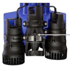
The switch-off point of the float switch for all types is at the height of the centre selvedge between upper and lower part of the aerator housing (see also marking on the side of the carrier frame).
