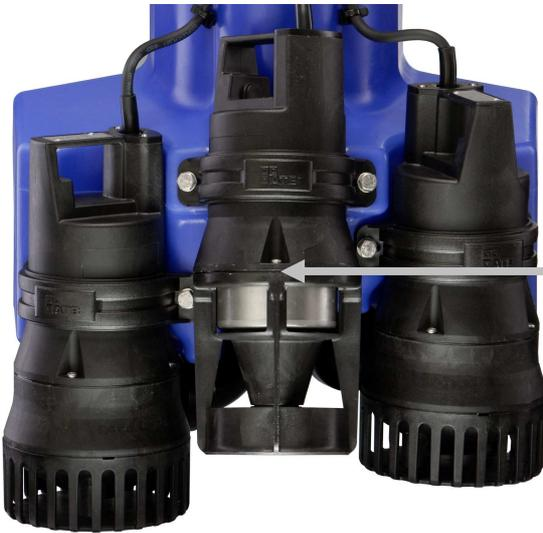
The switch-OFF point of the float switch (= SW1), with all types, is located at the height of the partition edge between upper and lower part of the aerator housing. The difference (=  $H_{W,min}$ ) between this point and the tank sole may not be undercut.
