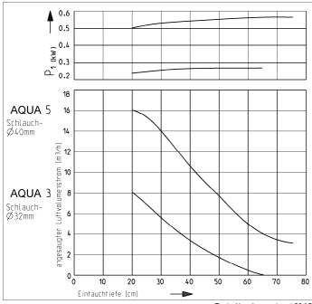
Tested in: clear water at 20 °C Tank surface: > 3 m Water depth: 1,5 m
